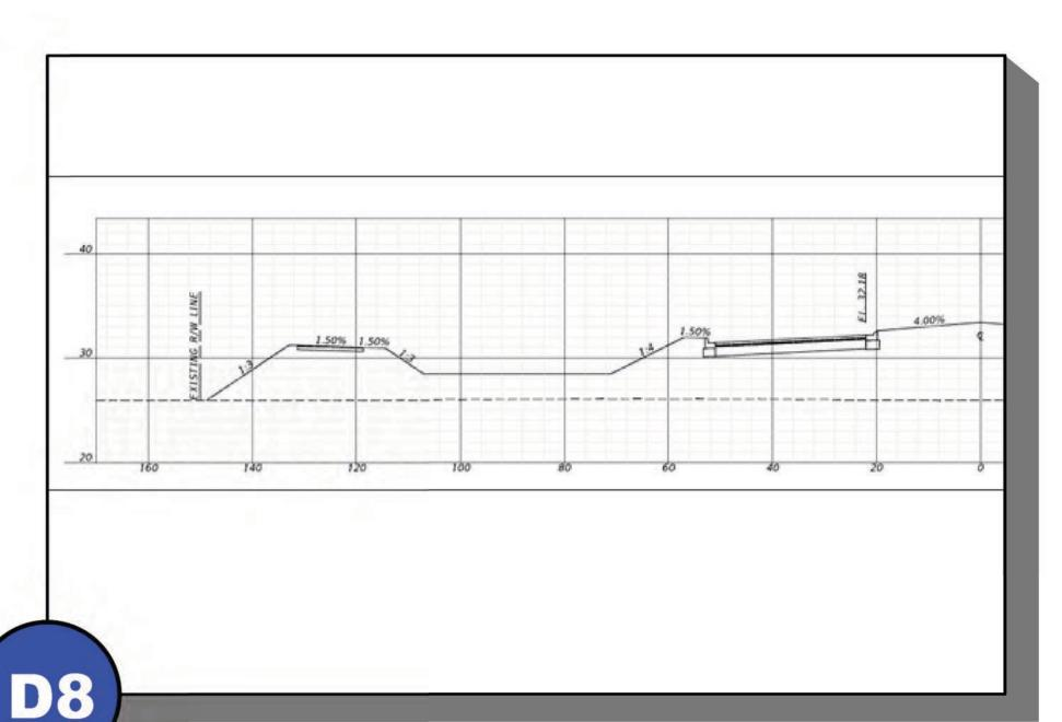
**Dry Treatment Ph3** Linear dry detention is being proposed for the entire length of roadway adjacent to the Jamerson Farms property. This will provide water quality treatment and quantity attenuation before it is ultimately discharged to the west.
