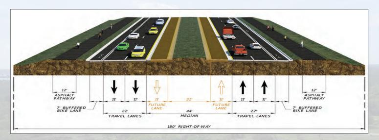
The Phase 2 improvements consist of a divided four-lane roadway, (expandable to six-lanes in the future), with closed drainage, 7-foot on-road bike lanes, some sidewalk, and multi-use paths in some areas, similar to the recently completed portion of Alico Road, east of Ben Hill Griffin Parkway.
